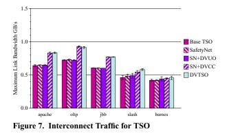
shows some unexpected speedups on *slash* when SafetyNet is added. With *slash*, SafetyNet slightly delays some writes, which can reduce lock contention and lead to a performance increase.
