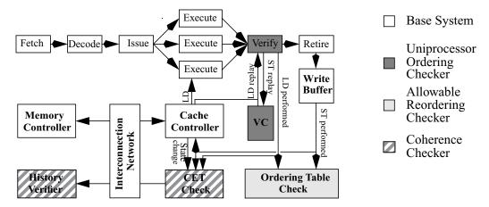
Figure 2. Simplified pipeline for DVMC. Single node shown. Several structures (memory, caches, MET,...) omitted for clarity.
