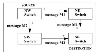
**Figure 1. Violating point-to-point order with adaptive routing.** The NW Switch sends Message M1 at time 1 and then message M2 at time 2 to the SE Switch. Message M2, however, arrives at time 3, which is before message M1 arrives at time 4.
