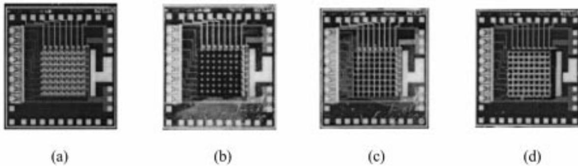
Fig. 3. Photomicrographs of  $8 \times 8$  array process: (a) circuit (b) thin-film P-i-N detector devices with linked layer bonded to planarized/via cut/metallized circuit (c) linking layer removed, (d) planarization/isolation, top via metal contact completed.
