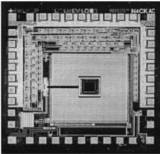
Fig. 4. Hybrid integrated OEIC with a thin-film resonant cavity-enhanced light-emitting diode bonded into the center of a Si CMOS BJT array. The analog transmitter and receiver circuitry and digital signal processing circuitry surround the detector.
