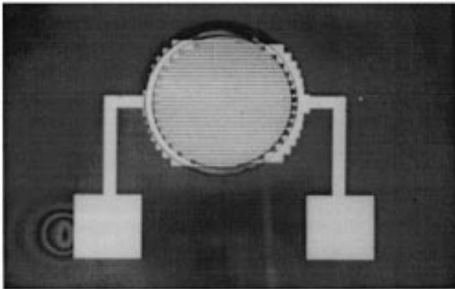
Fig. 2. Thin-film GaAs-based MSM bonded to silicon nitride-coated Si host substrate.
