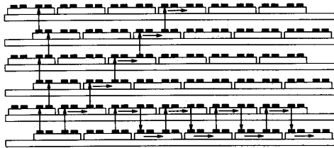
Fig. 4. Routing paths in an offset cube.
