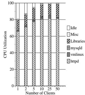
FIGURE 7. SlashCode: Utilization vs. # of Clients
