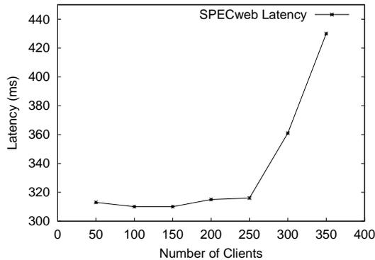
FIGURE 8. SPECweb: Latency vs. # of Clients
