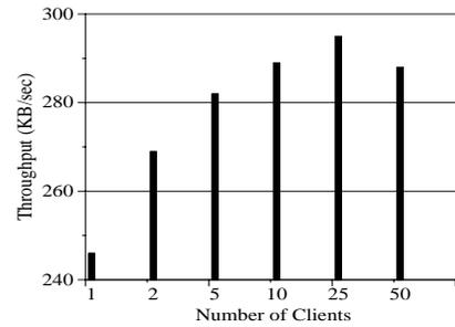
FIGURE 6. SlashCode: Throughput vs. # of Clients
