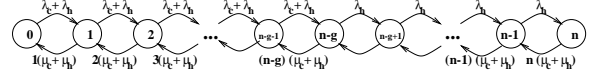
Figure 4. Birth-death process: n = MN - 1 (system working) or n = M(N - 1) - 1 (one base repeater down)
