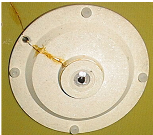
Figure 6. Bottom view of the Dewar showing the excitation coil that allows us to perform susceptibility measurements. The SQUID loop is located directly above the black epoxy window.
