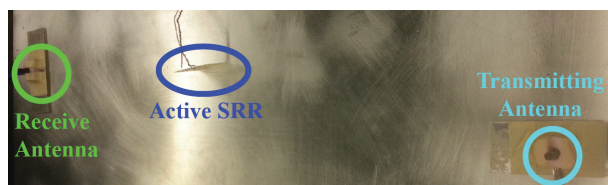
Fig. 9. Configuration and measurement setup for demonstrating the effectiveness of an SRR acting as a repeater. The SRR was 45 cm from both antennas.
