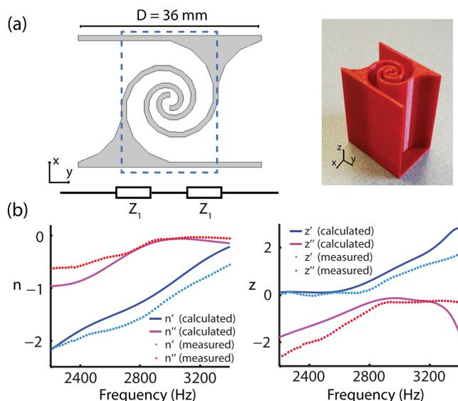
FIG. 2. Anisotropic spiral unit cell. (a) Geometry of the cross section of the unit cell, an equivalent transmission line diagram and a photograph of a 3D printed sample. (b) Experimentally measured and numerically retrieved refractive index and impedance.
