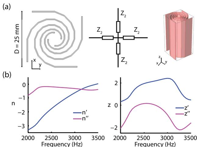
FIG. 3. Isotropic spiral unit cell. (a) Geometry of the cross section of the unit cell, an equivalent transmission line diagram and a computer generated 3D model. (b) Numerically retrieved refractive index and impedance.
