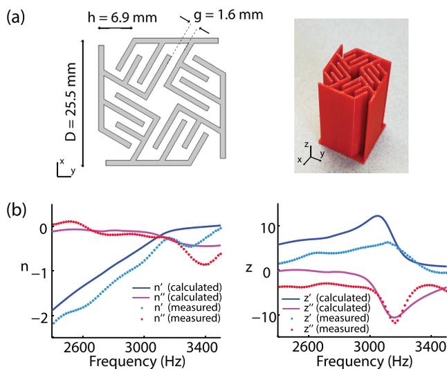
FIG. 1. Horn-port labyrinthine unit cell. (a) Cross sectional geometry and a photograph of a 3D printed sample. (b) Experimentally measured and calculated refractive index and impedance.
