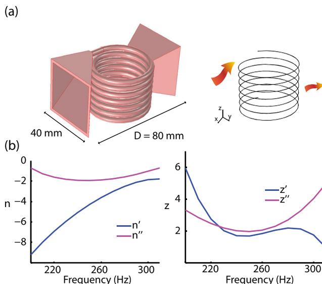
FIG. 5. Three-dimensional helical space-coiling unit cell (a) A computer generated 3D model and a schematic diagram of the propagation of acoustic wave inside the seven layer space coiling helical structure. (b) Numerically retrieved refractive index and impedance.
