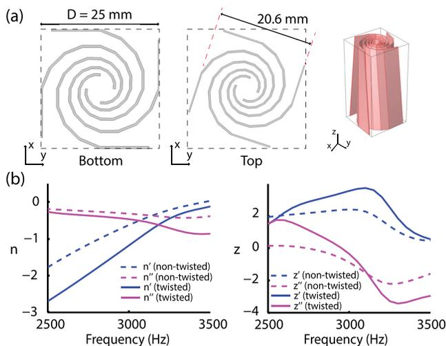
FIG. 4. Isotropic spiral unit cell with  $18^\circ$  twist along its height. (a) A computer generated 3D model. (b) Numerically retrieved refractive index and impedance.
