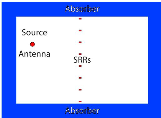
**Figure 6.** Geometry considered both for COMSOL simulations and imaging experiments. The eight SRRs form an array in the center of the domain, spaced 0.75 wavelengths apart. An absorber is used as a PML in simulations and to reduce the effects of external scatterers and interference in the experiments.
