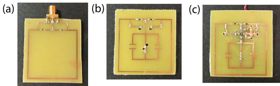
**Figure 3.** Photographs of fabricated PC metamaterials. (a) The simple direct RF connected metamaterial. (b) The passive, all-wireless metamaterial. (c) The active, DC bias connected metamaterial.
