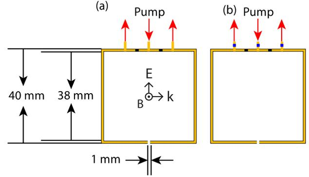
**Figure 1.** Schematic of PC SRR design. Black rectangles are the varactor diodes. Dimensions are shown along with signal paths and polarization. The signal path for the pump leads to a direct cable connection with an SMA adaptor. (a) The simple RF connected element. (b) The simple RF connected element with matching network.
