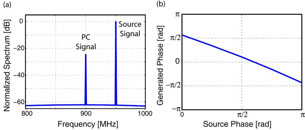
**Figure 4.** Numerical study of the mixing process. (a) Generated signal amplitude relative to the source signal. (b) Phase of the generated signal as a function of the source signal phase. A positive change in the source phase yields a negative change in the generated signal phase, indicating that the generated signal is PC.
