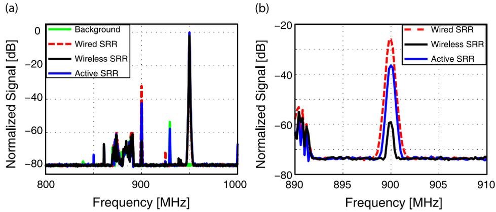
**Figure 5.** Measured spectra for four cases. Solid green is background signal levels (no equipment on). Dashed red is the simple RF connected metamaterial. Solid black is the all-wireless metamaterial. Solid blue is the active metamaterial. (a) Full measured spectrum normalized to the source signal (at 950 MHz). (b) Zoom on the PC signal normalized to the incident source signal to determine PC signal generation efficiency.
