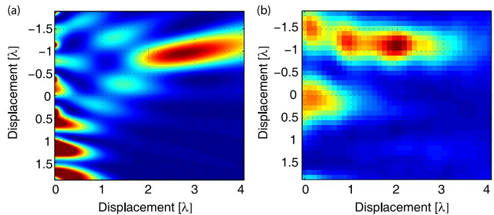
**Figure 9.** Simulated and measured field patterns for the off-axis source experiment. (a) Simulated normalized  $|E|$ , with the scale in wavelengths. (b) Measured normalized  $|E|$ , with the scale in wavelengths.
