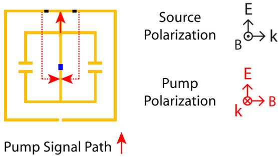
**Figure 2.** Schematic of the wireless metamaterial design. Black rectangles are the varactor diodes. The blue rectangle provides a load to harvest voltage from the ELC section. The pump signal path is shown by red arrows. The dashed arrows are on the underside of the dielectric using vias. Appropriate polarizations for the source and pump are shown.
