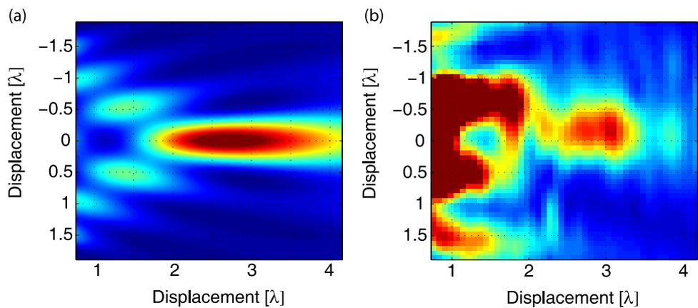
**Figure 8.** Simulated and measured field patterns for the centered source experiment. (a) Simulated normalized  $|E|$ , with the scale in wavelengths. (b) Measured normalized  $|E|$ , with the scale in wavelengths.
