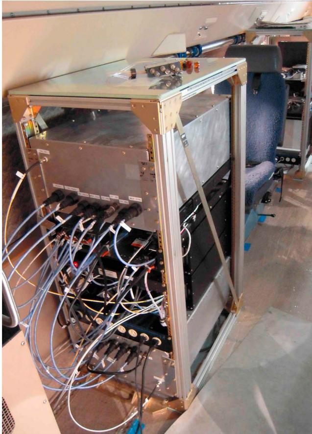
**Figure 1.** ADELE installed in the GV. The aluminum boxes at top and bottom are the sensor heads; the two computers are the black boxes in the middle of the rack.
