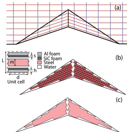
FIG. 2. (Color online) Ground cloak design. (a) Contour plot of mapping functions  $u(x)$  and  $v(x, y)$ ; (b) structure of cloak composed of arrays of discrete unit cells. The dimensions of the unit cell elements are  $L = 50$  mm,  $d = 47.5$  mm,  $m = 14.7$  mm,  $s = 1.8$  mm, and  $h = 12.38$  mm; (c) ideal cloak made of the homogeneous continuous and anisotropic material that is implemented through the metamaterial depicted at (b).
