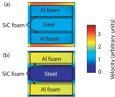
FIG. 5. (Color online) Particle velocity inside the solid inclusions for two types of unit cells: (a) foam and steel inclusions are in direct contact; (b) foam and steel inclusions are isolated by a narrow water channel. This cell was used to generate the cloak.
