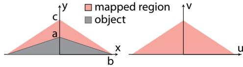
FIG. 1. (Color online) Principle behind the ground cloak. A mapping between the real,  $xy$ , and virtual,  $uv$ , spaces is chosen such that the object in the real space is flattened, i.e., mapped to the ground plane, in the virtual space
