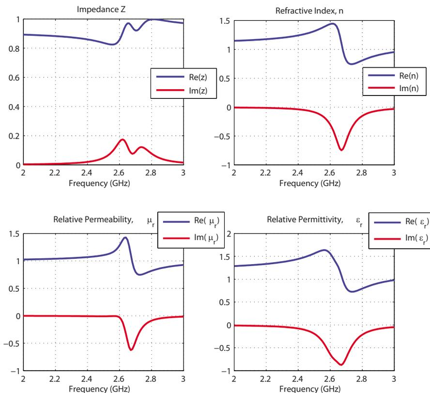
FIG. 4. (Color online) ELC-SRR retrievals. Permeability ( $\mu_r$ ) and permittivity ( $\epsilon_r$ ) have similar Lorentzian resonances around 2.67 GHz.  $Z$  is therefore near unity and  $\text{Im}(n)$  is large.
