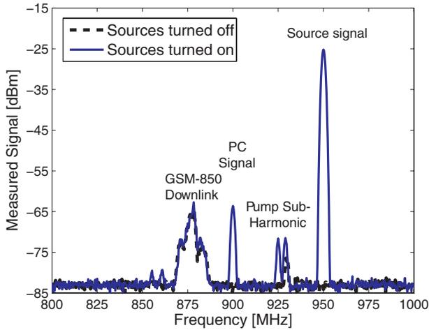
FIG. 2 (color online). Data from spectrum analyzer for background signal (dashed black) and pump and source signals switched on (solid blue). Notable frequencies include 900 MHz ( $f_{pc}$ ), 950 MHz ( $f_{source}$ ), and 1850 MHz (not shown).
