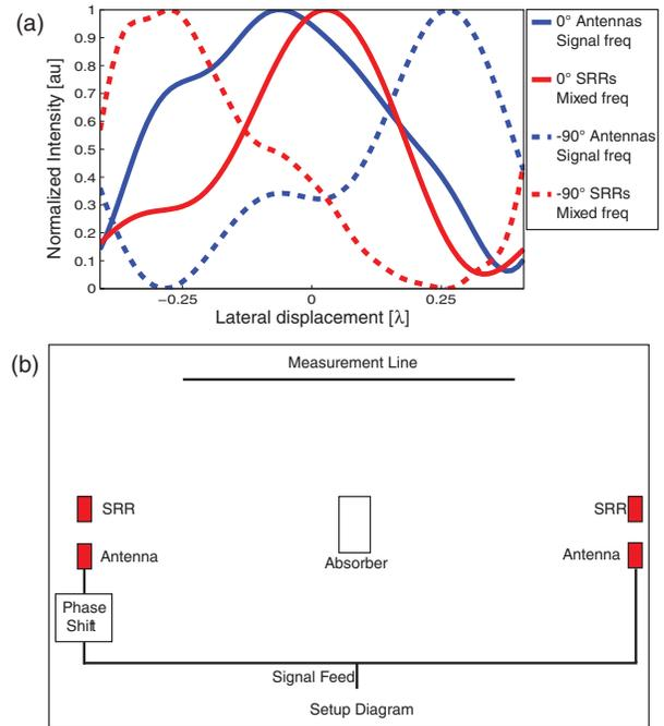
FIG. 3 (color online). (a) Interference pattern for in-phase antennas at  $f_{signal}$  (solid blue),  $-90^\circ$  out-of-phase antennas at  $f_{signal}$  (dashed blue), in-phase SRRs at  $f_{mixed}$  (solid red),  $-90^\circ$  out-of-phase SRRs at  $f_{mixed}$  (dashed red). (b) Schematic of setup (to scale). Antennas were fed at  $f_{signal}$  with both  $0^\circ$  and  $-90^\circ$  phase shifts. The absorber was used to isolate antennas and SRRs.
