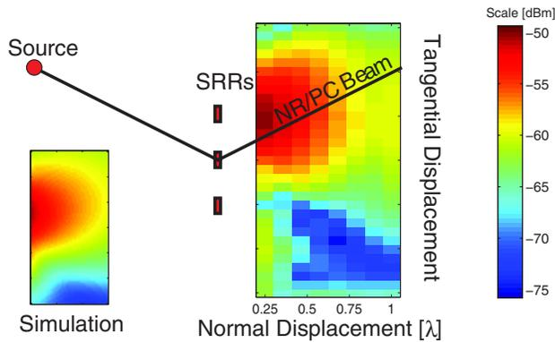
FIG. 4 (color online). Measured  $abs(E)_{dBm}$  and experimental setup. The setup is approximately to scale. The source radiates from the upper left in the figure and SRRs produce a mixed signal at  $f_{pc}$ . The inset shows calculated results, exhibiting good agreement. The measurements show that the beam negatively refracts.
