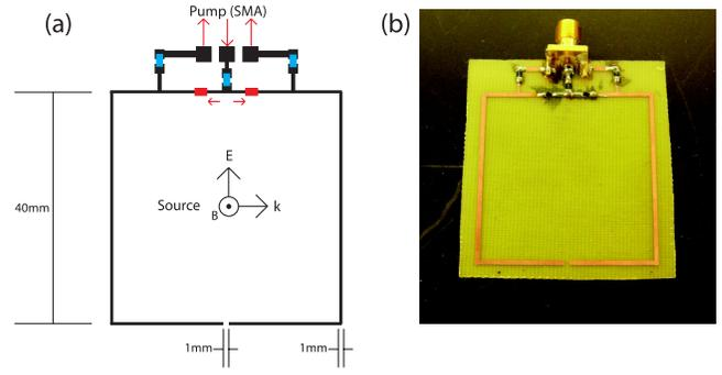
FIG. 1 (color online). (a) Layout of SRR element. Red (horizontal) elements are varactor diodes and blue (vertical) elements are isolation resistors. (b) Photo of fabricated SRR element.
