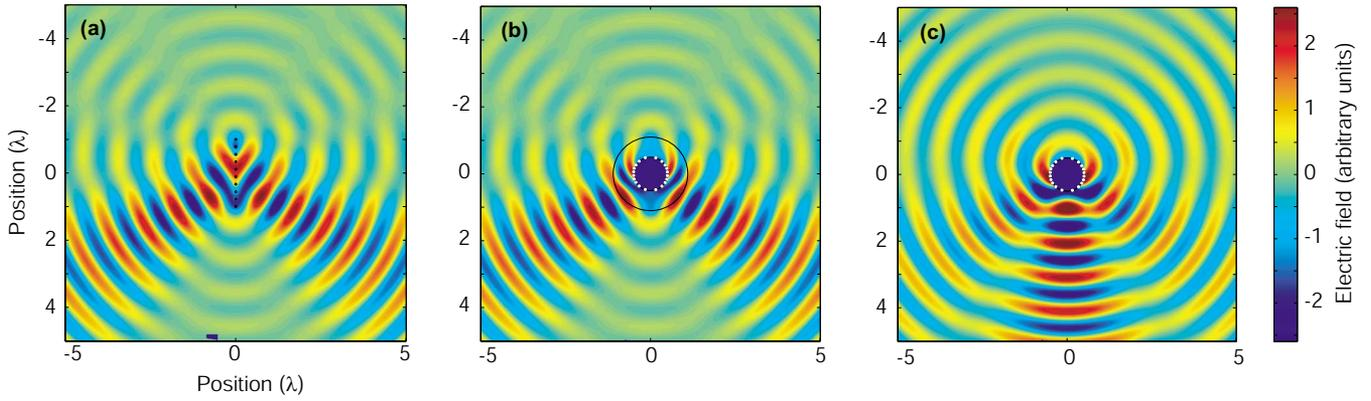
FIG. 2. (Color online) (a) Electric field produced by a phased array made of ten line sources spanning a length of  $2\lambda$ , designed to radiate in free space at an angle of  $30^\circ$ ; (b) Transformed phased array modified under geometrical constraints. The shell between the two cylinders is made of an inhomogeneous material designed using coordinate transformations; (c) Electric field in the absence of the shell.
