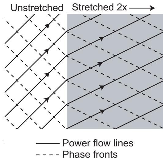
**Figure 1.** The deformation of power flow lines and phase fronts for a general uniform plane wave after a linear coordinate transformation in one direction. This deformation is the same for all types of waves (electromagnetic, acoustic, etc).
