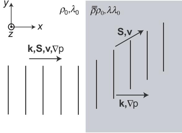
**Figure 4.** Schematic of an acoustic beam normally incident on a beam shifting material defined by an  $x$  dependent shift of the  $y$ -coordinate. The relationship between the  $\mathbf{v}$  and  $\nabla p$  vectors, the beam direction and the wave vector are shown for both materials.
