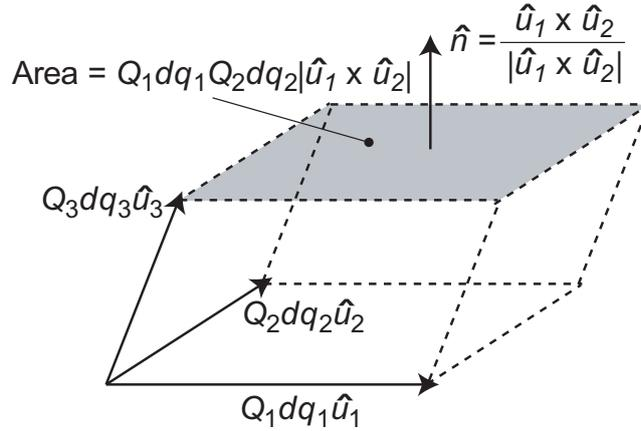
**Figure 3.** The parallelepiped that defines an infinitesimal volume in the transformed coordinates. The area and unit normal of each face enters in the calculation of the net flux of a vector out of this volume.
