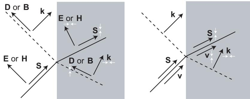
**Figure 2.** The transformation of vectors in electromagnetic (left) and acoustic or compressional elastodynamic (right). The white converging arrows denote which component of each vector is compressed by the coordinate transformation.
