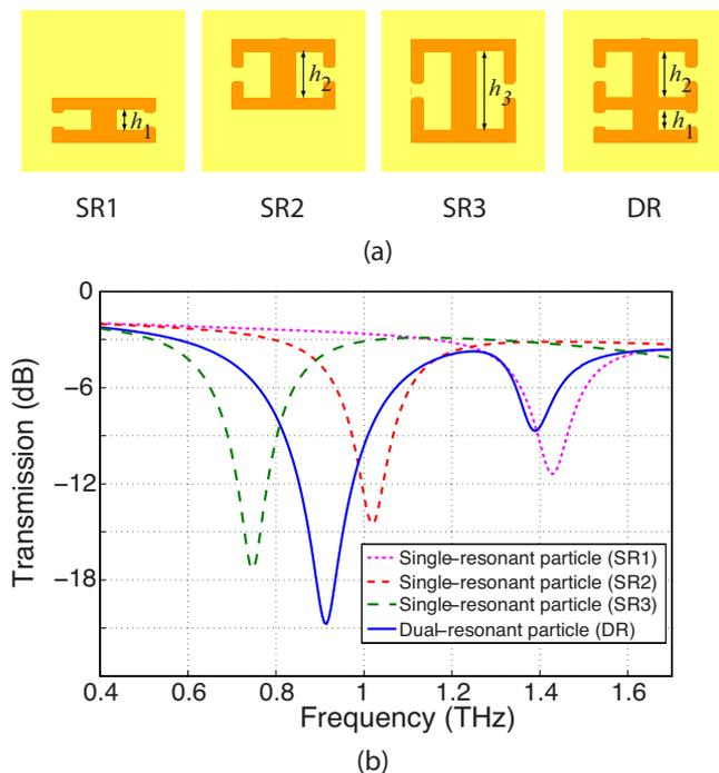
FIG. 3. (Color online) (a) Single-resonant particles SR1, SR2, SR3, and dual-resonant particle DR ( $h_1=6\ \mu\text{m}$ ,  $h_2=14\ \mu\text{m}$ , and  $h_3=24\ \mu\text{m}$ ). (b) Calculated transmission of the metamaterial composed of SR1, SR2, SR3 (pink, red, and green dashed lines, respectively), and DR (blue solid line).
