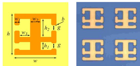
FIG. 1. (Color online) (Left) designed unit cell, with geometries:  $h=w=32\ \mu\text{m}$ ,  $w_1=4\ \mu\text{m}$ ,  $w_2=8\ \mu\text{m}$ ,  $w_3=8\ \mu\text{m}$ ,  $h_1=8\ \mu\text{m}$ ,  $h_2=14\ \mu\text{m}$ ,  $g=4\ \mu\text{m}$ , and  $b=0.8\ \mu\text{m}$ . (Right) Photomicrograph of the fabricated sample. The lattice constant of the unit cell is 50  $\mu\text{m}$ .
