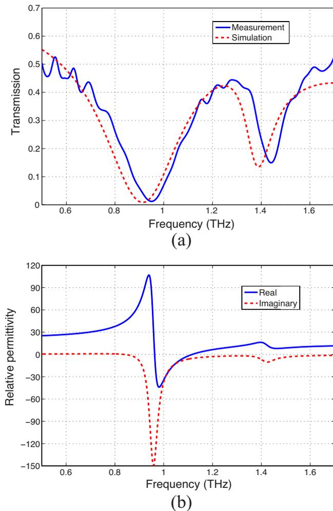
FIG. 2. (Color online) (a) Calculated (blue line) and measured (red line) transmissions of the metamaterial sample. (b) Retrieved permittivity of the metamaterial layer.
