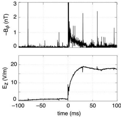
**Figure 1.** Unfiltered  $B_\phi$  and  $E_z$  for a stroke containing a continuing current signature in both fields, namely a slow increase in  $E$  and an elevated  $B$  following the return stroke.
