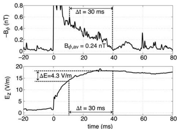
**Figure 4.** Measured  $B_\phi$  and  $E_z$  versus time for a +19.6-kA stroke 70.7 km from the sensors on 15 July 2005 at 02:02:07.635 UT.
