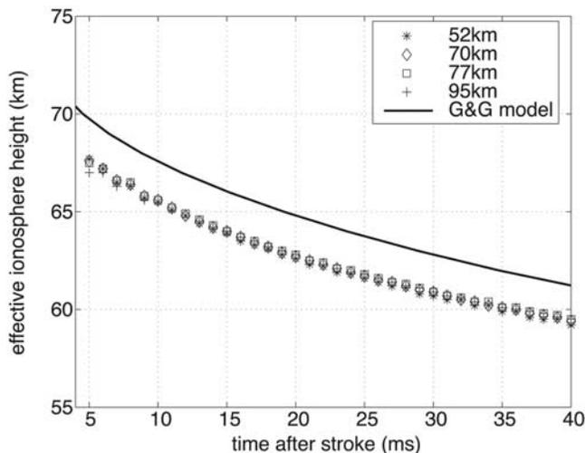
**Figure 3.** Effective ionosphere height versus time extracted from FDTD simulations compared with the approximate analytical approach of *Greifinger and Greifinger* [1976].
