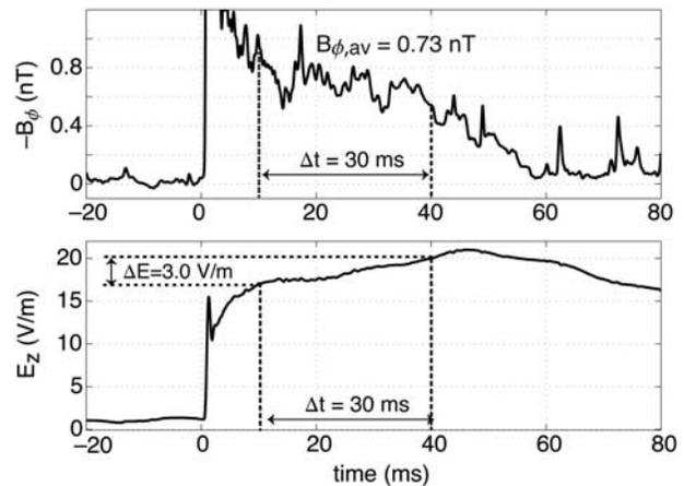
**Figure 6.** Measured  $B_\phi$  and  $E_z$  versus time for a +71.8-kA stroke 95.8 km from the sensors on 15 July 2005 at 03:43:10.870 UT.
