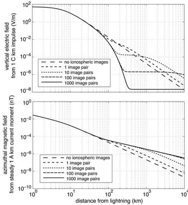
**Figure 2.** Computed electrostatic (top) and magnetostatic (bottom) fields versus distance for different numbers of ionospheric image pairs.
