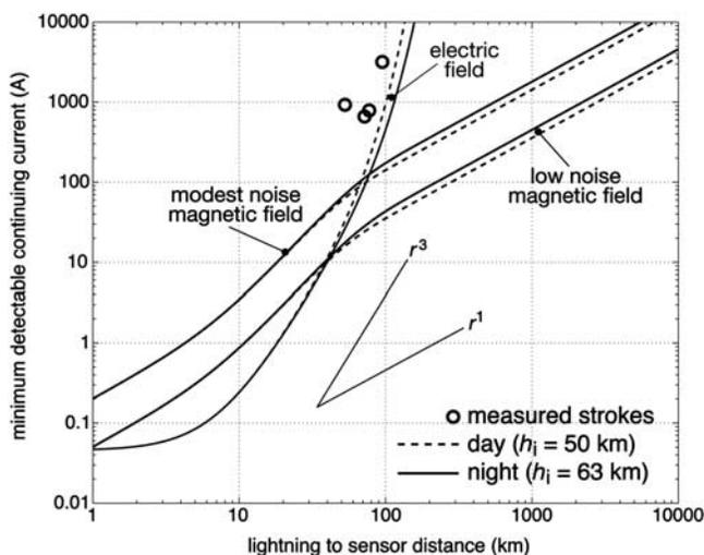
**Figure 7.** Minimum detectable continuing current for different sensors vs. distance to sensor. Plotted for reference are  $r^3$  and  $r^1$  lines, and the circles show the measured continuing current and range for the 4 events analyzed here.
