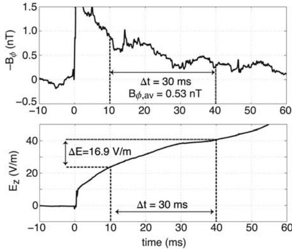
**Figure 5.** Measured  $B_\phi$  and  $E_z$  versus time for a +22.8-kA stroke 52.1 km from the sensors on 15 July 2005 at 02:05:34.031 UT.
