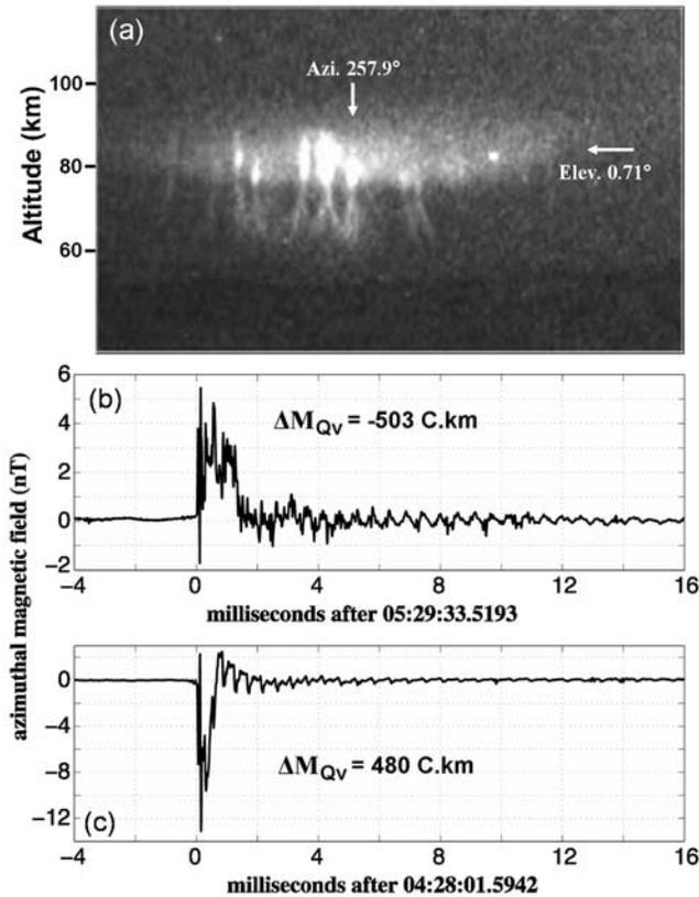
**Figure 2.** (a) Enlarged ( $6^\circ \times 4^\circ$ ) image of the negative event at 05:29:33.522 UT showing a well developed sprite-halo with streamers. (b) The ELF/VLF azimuthal magnetic field ( $B_\phi$ ) waveform associated with this event. (c) The  $B_\phi$  waveform of a sprite-halo (Figure 3c) produced by a positive CG of similar  $\Delta M_{QV}$ .
