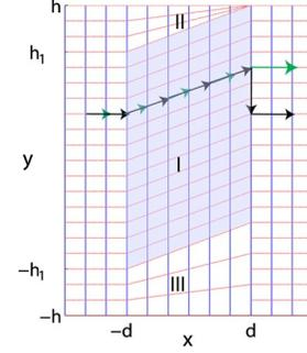
FIG. 1 (color online). Linear spatial coordinate transformation of a parallel beam shifter.
