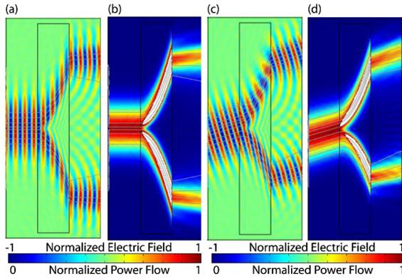
FIG. 4 (color online). Electric field distribution (color map), power flow lines (gray) [(a) and (c)] and power flow [(b) and (d)] of a beam splitter for diffracting plane waves with shift parameters (a)–(b)  $|a| = 15$  for perpendicular incident waves and (c)–(d)  $|a| = 12$  for oblique incidence. The power flow color maps are saturated for the sake of contrast enhancement.
