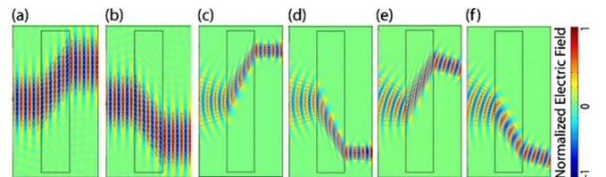
FIG. 3 (color online). Electric field distribution (color map) and power flow lines (gray) of a parallel beam shifter for diffracting plane waves with shift parameters (a)  $a = 1.8$ , (b)  $a = -1.8$ , for a convergent beam under perpendicular incidence with (c)  $a = 2$ , (d)  $a = -2$  and for oblique incidence with (e)  $a = 2$  and (f)  $a = -1.2$ .
