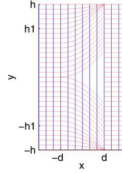
FIG. 2 (color online). Nonlinear spatial coordinate transformation of second order for a beam divider.
