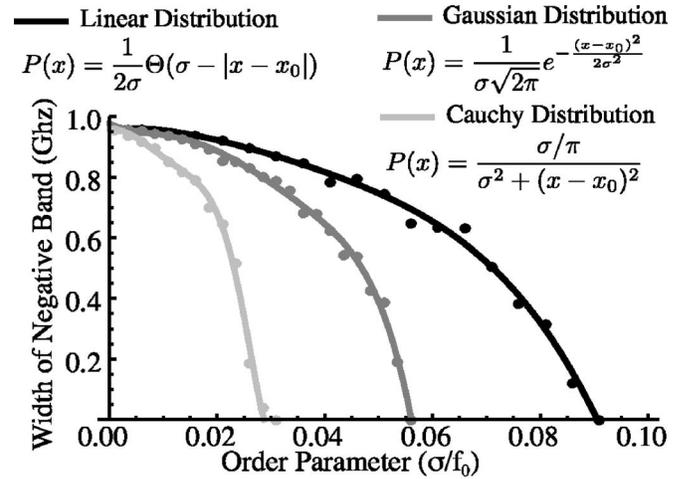
FIG. 3. For a characteristic SRR structure in our experiment ( $f_0=12.5$  GHz,  $Q=78$ ,  $F=0.14$ ), a numerical calculation of the width of negative region as a function of disorder introduced is shown for linear, Gaussian, and Cauchy distributions.
