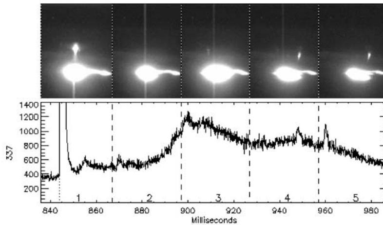
**Figure 1.** Example of a sprite observation on September 23, 2005 where a total of four sprites occur immediately after the parent lightning and with 62, 104, and 116 msec delay, respectively. The long elevated signal in the photometer and the long lasting brightness of the lightning in the images are caused by the continuing current after the +CG stroke.
