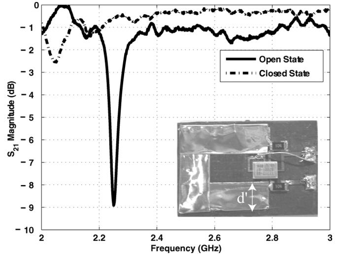
Fig. 6. Open and closed switch responses of the parallel circuit configuration. The resonant response of our ring from Fig. 5 with the gap capacitance  $C$  shorted is at the edge of the waveguide passband, and so we decreased  $L$  to raise  $f_0$  by increasing the trace thickness to  $d' = 5.5$  mm.
