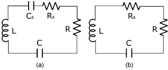
Fig. 1. Equivalent circuit of the loop with the MEMS switch used in a series configuration. The open switch (a) introduces a capacitance  $C_s$ , whereas the switch resistance  $R_s$  is present in both the open and closed (b) states.
