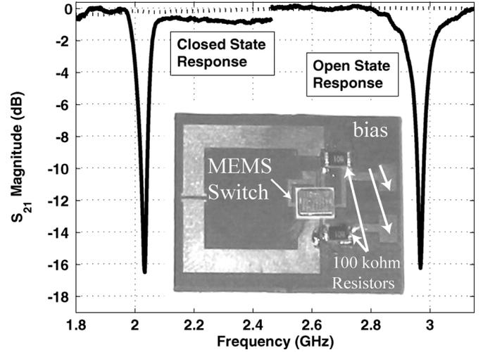
Fig. 5. Open and closed switch responses for the series resonant circuit, where  $Q_{\text{closed}} \approx 150$  and  $Q_{\text{open}} \approx 250$ , and the dashed plot shows  $S_{21}$  for the unloaded waveguide. Also shown are the pads for the dc bias and 100 k $\Omega$  resistors used for isolation of the external dc voltage source.
