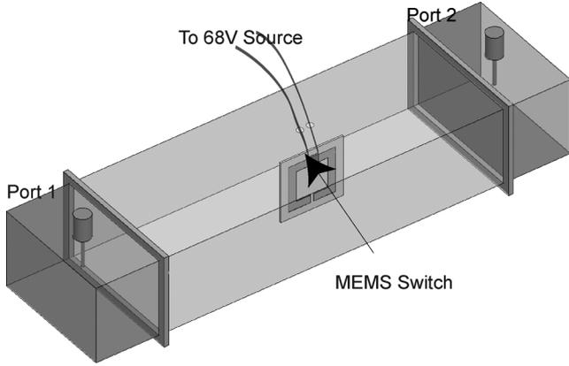
Fig. 4. Diagram of the dual-state switchable ring placed inside the WR-340 waveguide.
