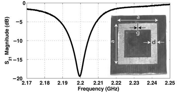
Fig. 3. The resonant copper ring on Rogers Duroid substrate ( $\epsilon_r = 2.2$ ,  $\tan \delta = 0.0009$ ) in the absence of the MEMS switch, with  $S_{21}$  measurements made in the WR-340 waveguide ( $a = 16$  mm,  $d = 2.5$  mm, and  $g = 0.3$  mm). It was designed to be resonant at 2.2 GHz, and experimental transmission measurements placed very close to this frequency, where measured  $Q \approx 600$ .
