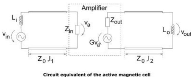
**Figure 2** Circuit equivalent of the active magnetic cell
