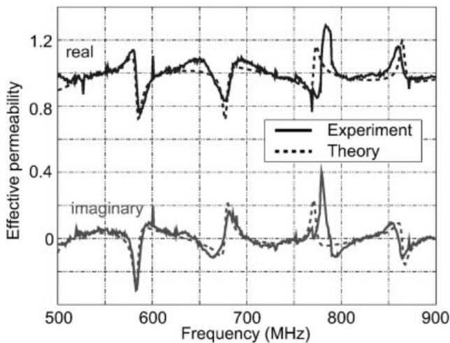
**Figure 5** Match between the theoretical and retrieved permeability for a unit cell containing the minicircuits ZHL2010 amplifier connected to the Maxim MAX2472 voltage buffer
