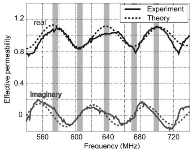
**Figure 4** Effective permeability retrieved from measurements for a unit cell containing an 1W1000 amplifier. There are frequencies with almost no dispersion and zero loss (the shadowed regions)
