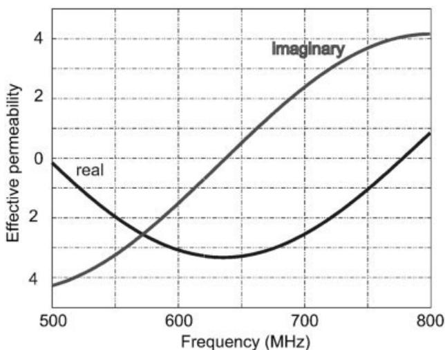
**Figure 6** Theoretically achievable effective permeability in a metamaterial composed of active unit cells, provided the right amplifier is used
