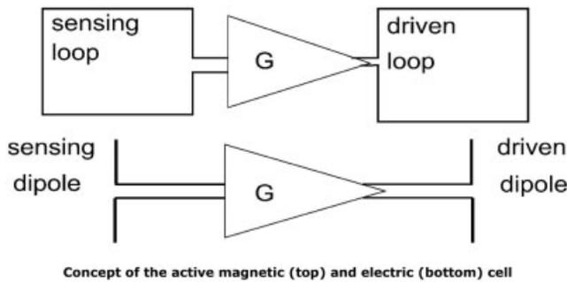
**Figure 1** Concept of the active magnetic (top) and electric (bottom) cell
