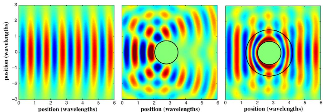
**Figure 2.** Left panel: The acoustic pressure  $p$  in the absence of a scatterer. Middle: The acoustic pressure with an incompressible cylindrical scatterer. Right panel: The acoustic pressure with the same scatterer surrounded by the cloaking shell described in the text.
