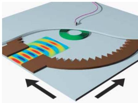
**Fig. 3.** Cutaway view of the planar waveguide apparatus. Microwaves (red and yellow patterns) are introduced by means of a coaxial-to-waveguide transition (not shown) attached to the lower plate (lined with a circular sawtooth-shaped microwave absorber). An antenna mounted in the fixed upper plate measures the phase and amplitude of the electric field. To perform field maps, we stepped the lower plate in the lateral directions (black arrows).
