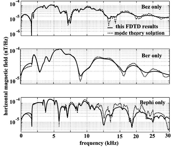
Fig. 5. Comparison between the numerical simulation results of this FDTD model and mode theory solutions. Upper panel: Earth's magnetic field is vertical; middle panel: Earth's magnetic field is in *r* direction; lower panel: Earth's magnetic field is in  $\phi$  direction.
