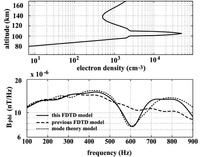
Fig. 9. Numerical simulation results with the presence of an  $E_s$  layer. Upper panel: the electron density profile with an  $E_s$  layer; lower panel: the comparison between the simulation results of the previous FDTD model with the simple conductor approximation, this FDTD model, and the mode theory model. The spatial grid size is 0.5 km for the FDTD models.
