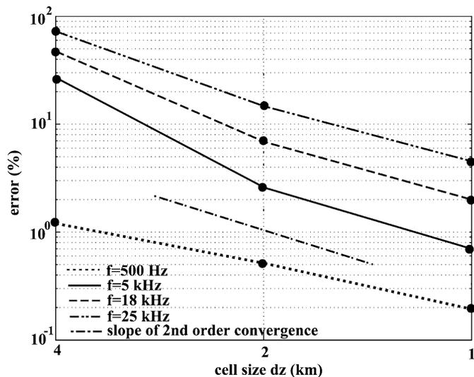
Fig. 10. Convergence of solution of this FDTD model solutions: the absolute value of the relative errors of this FDTD model with different cell sizes (0.5, 1, 2, and 4 km). The solution of  $\Delta z = 0.5$  km case is regarded as the reference value.
