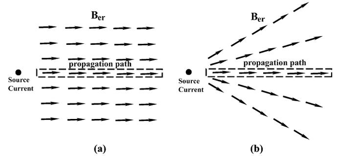
Fig. 3. Diagrams of Earth's magnetic field (only  $r$  component is shown): (a) 3-D model and (b) 2-D cylindrical model.
