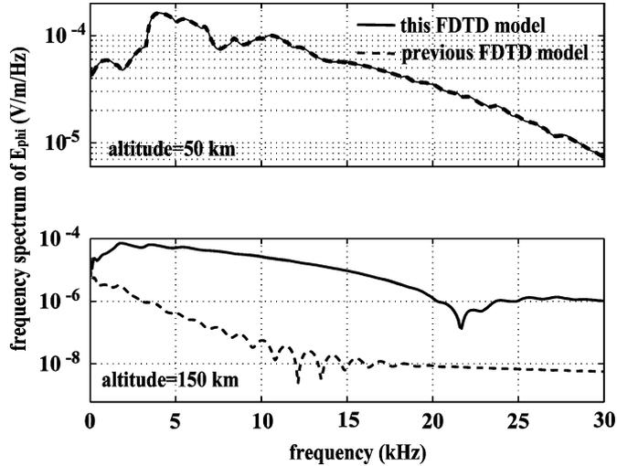
Fig. 8. Comparison between simulation results of this FDTD model and the previous model with the simple conductor approximation at low and high altitudes. Upper panel: the altitude is 50 km; Lower panel: the altitude is 150 km.
