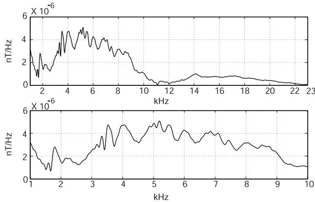
**Figure 2.** Average spheric spectrum from 10 sferics with later-time filtering and its fine structure.
