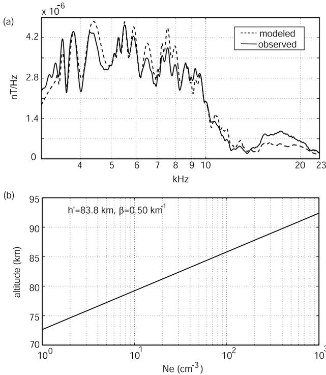
**Figure 3.** (a) Observed and best fit modeled sferic spectra on a frequency scale highlighting the fine structure agreement. (b) Measured  $D$  region electron density.
