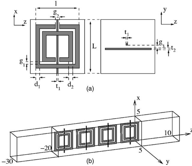
FIG. 1. (a) Unit cell:  $L=5$  mm,  $l=4$  mm,  $d_1=0.33$  mm,  $d_2=0.33$  mm,  $g_1=0.1$  mm,  $g_2=0.3$  mm,  $g_3=0.2$  mm,  $t_1=0.02$  mm, and  $t_2=0.02$  mm; (b) setup: four cells in the propagation direction; PEC boundary conditions on the  $x=0$  mm and  $x=5$  mm planes; PMC boundary conditions on the  $y=0$  mm and  $y=5$  mm; wave ports at  $z=-30$  mm and  $z=10$  mm.
