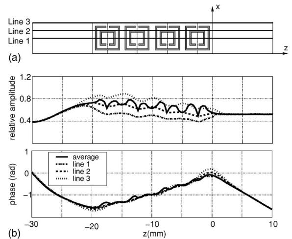
FIG. 4. (a) The electric field is measured along three lines given by the following equations:  $x=2.5$  mm,  $y=0$  mm (line 1);  $x=3.75$  mm,  $y=0$  mm (line 2);  $x=5$  mm,  $y=0$  mm (line 3). (b) Electric field (amplitude and phase) averaged over the transverse  $xy$  plane, and the electric field along the three sampling lines.
