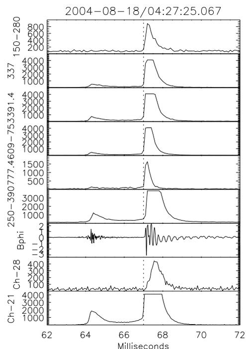
**Figure 2.** Photometer observations during the elve observed on August 18, 2004 (Figure 1a). The top six panels show the SP data in instrument counts with their pass bands. The following panel gives the azimuthal (Bphi) component of the VLF radiated magnetic field. The bottom two panels give two selected AP-channels with Ch-21 centered at the low-altitude lightning, and Ch-28 centered at the high altitude elve.
