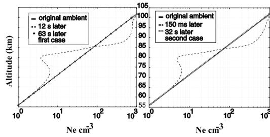
**Figure 3.** (left) The measured  $D$  region electron density profiles during the perturbation on July 25, 2000, from 03:26–03:29 UT. (right) The measured  $D$  region electron density profiles during the perturbation on June 30, 2000, from 04:21–04:23 UT.
