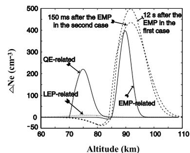
**Figure 4.** The resulting electron density change caused by the big lightning on July 25, 2000 in the first case and that on June 30, 2000 in the second case and compared to the qualitative shape of  $\Delta N$  produced by QE-related, EMP-related and LEP-related model.
