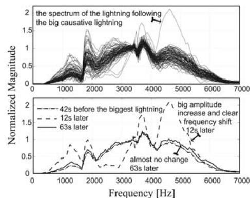
**Figure 2.** (top) Spectra of 100 lightning discharges with good SNR from 03:04 UT to 03:38 UT on July 25, 2000 at the same location. (bottom) Spectra of 3 probe strokes from 03:26–03:29 UT on July 25, 2000 at the same source location.
