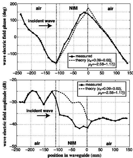
FIG. 4. Measured electric field phase (top) and amplitude (bottom) spatial distributions. The reversed phase gradient in the NIM confirms oppositely directed phase velocity and energy flow. Also shown are theoretical fits to the data used to measure the effective bulk permittivity and permeability of the NIM.
