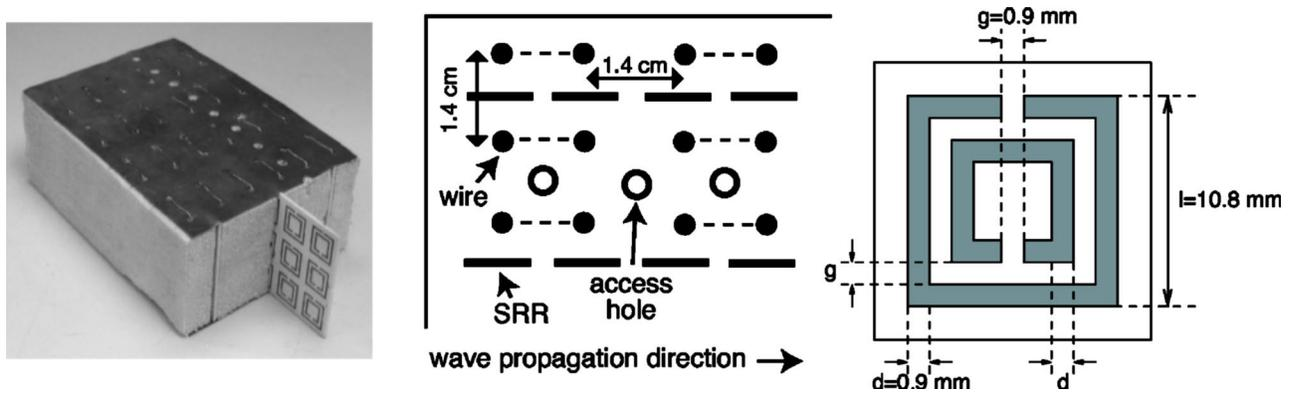
FIG. 2. Left: a photograph of the NIM slab used in these experiments. Middle: a plan view of the NIM slab. Right: dimensions of an individual SRR in the slab.
