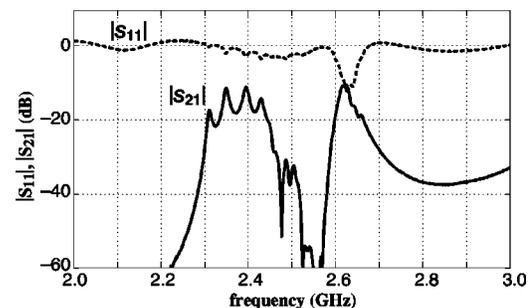
FIG. 3. Measured  $S$  parameters for the three slab waveguide configuration.
