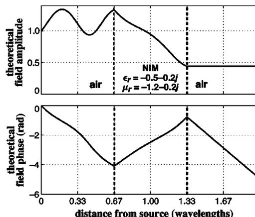
FIG. 1. Theoretical plots of the field phase and amplitude distributions in a representative normal incidence three slab (air/NIM/air) problem. The assumed relative NIM parameters are shown. The reversed phase gradient in the NIM is the targeted measurement and would confirm negative index behavior.
