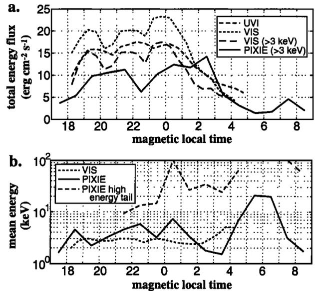
**Figure 2.** Energy parameters extracted from the three imagers between 0440 and 0445 UT. a: Total energy flux as a function of local time. b: Mean electron energy and high energy tail e-folding energy as a function of local time.
