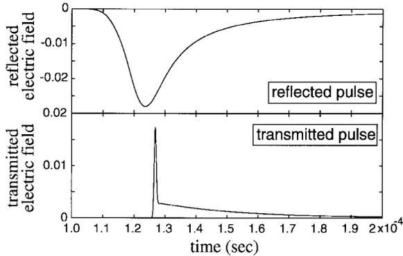
Fig. 8. Plots of the reference solution reflected and transmitted pulses for the  $\nu\Delta t \approx 1$  problem.
