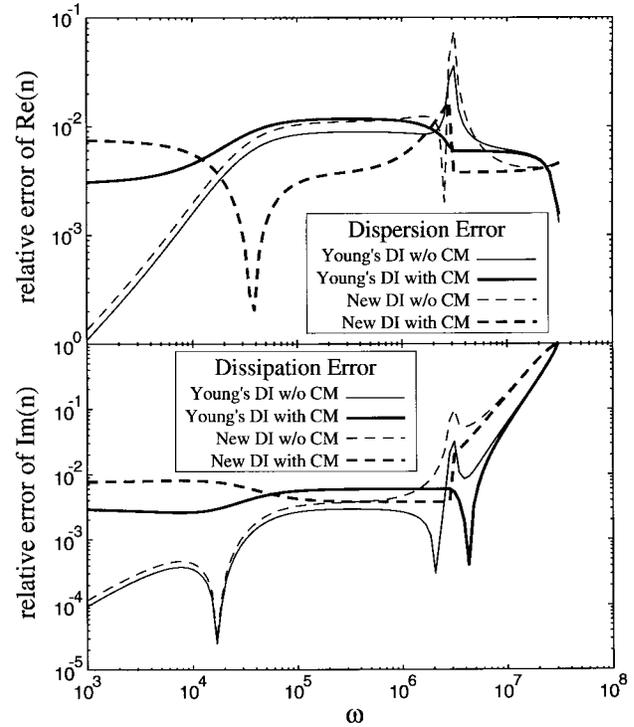
Fig. 4. A plot of dispersion and dissipation error versus  $\omega$  for Young's DI and the new DI methods with and without cutoff modification. Cutoff modification reduces the upward spikes near the plasma frequency at the expense of reduced accuracy at lower frequencies.
